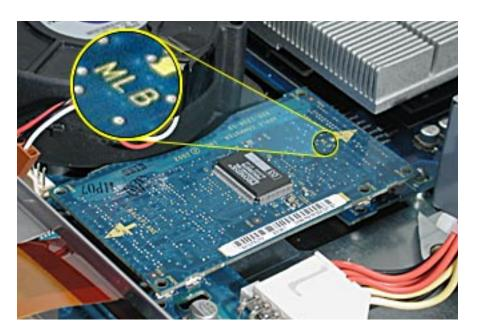
8. Reinstall the two ATA controller clips.
